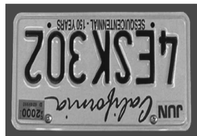
Inverted image, normal with Newtonians & as viewed with eyepiece directly in a refractor.
